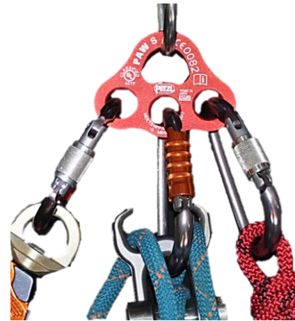
Figure 53- Rigging Plate. Keeps multiple connections organized.
