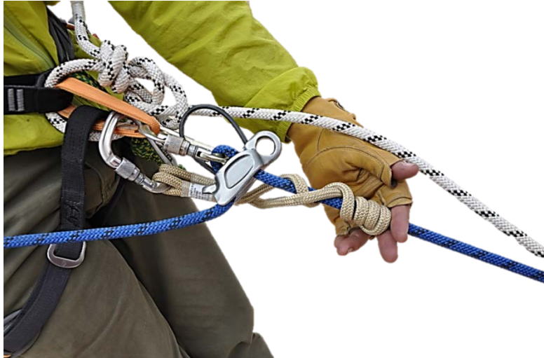
Figure 145- VT Prusik as autoblock for rappelling. In this configuration it can be tended and released easily.
