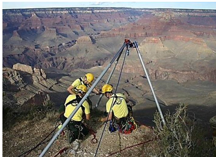
Figure 166- AZ Vortex Artificial High Directional in easel A-frame configuration.
