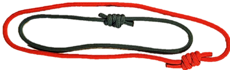
Figure 98- Tandem Prusiks constructed with contrasting colored 8mm cord for easy visual identification.
