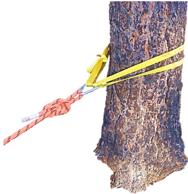
Figure 110- Basket Hitch Anchor with a triangular screw link employed at the collection point.
